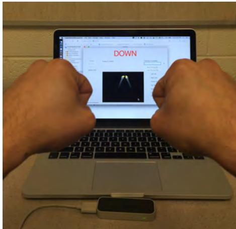
After defining the gesture language we used a Parrot Bebop quadcopter along with Leap Motion - a computer hardware sensor device that supports hand and finger motions as input, analogous to a mouse, but requiring no hand contact or touching (Figure 7) for the purpose of this research.
