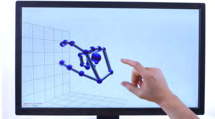
The sensor connects to a computer using an USB port. The computer will gather raw data from the sensor and the software system embedded in the computer will decide based on the gesture type which command it should send to the quadcopter (Figure 8).
