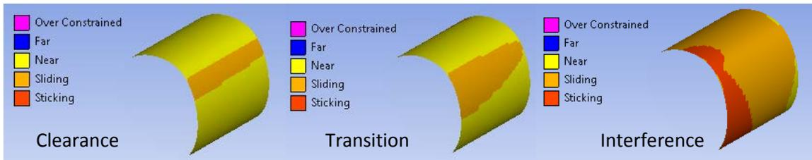
Figure 66: Contact status in P3G profile for loading case 2
