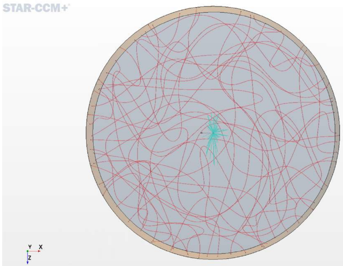
Figure 62. Average drug dispersion from cannula for 12 mm tissue and 20° x 13 mm Lg. cannula (a) top view.
